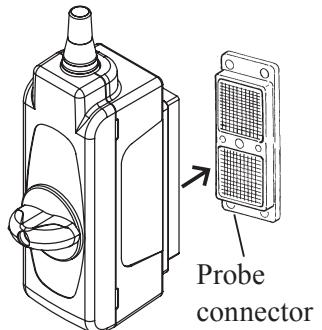
1. Turn the connector lock lever to align the
