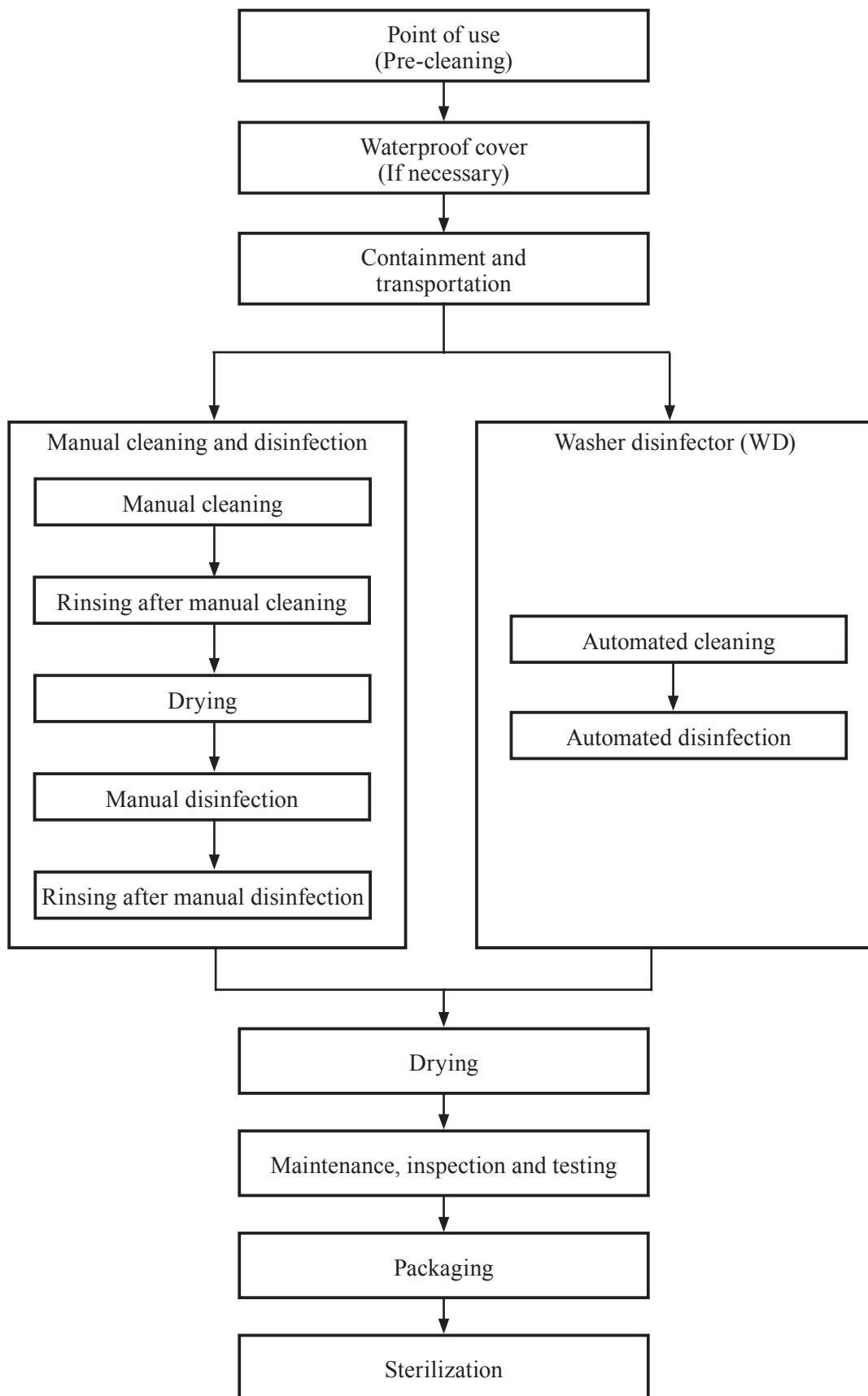
NOTE: Only the accessories are compatible with automated reprocessing according to the flowchart above.
