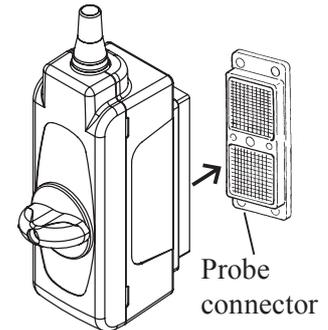
1. Turn the connector lock lever to align the ○ mark on the lever with the RELEASE position.
