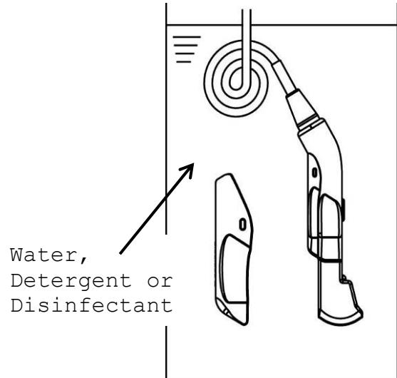
Fig. 18 Immersion of the probe and the Attachment.
