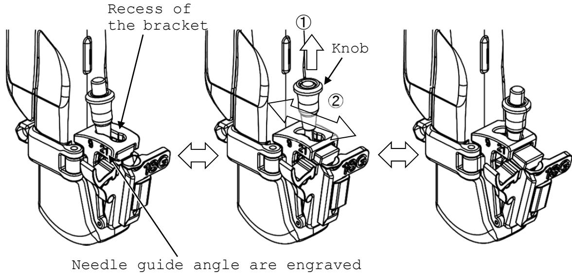
Fig. 17 Setting the needle guide angle
