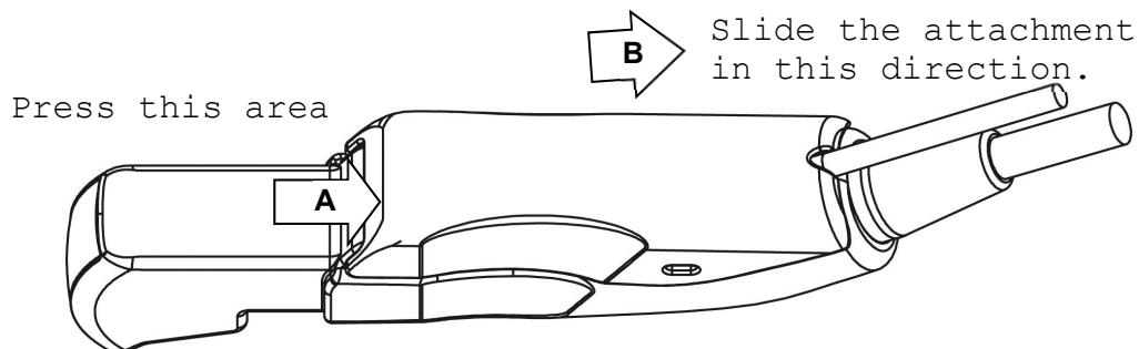
Fig. 8 How to release the attachment from the probe
