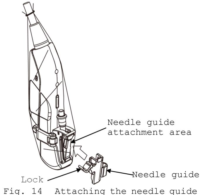
Fig. 14 Attaching the needle guide
