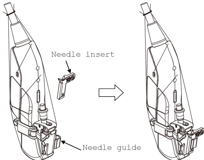
Fig. 16 Attaching the needle insert
