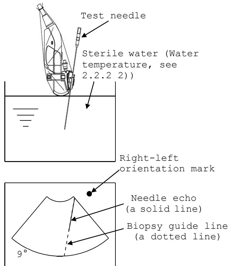
Fig. 2 Echo image of the test needle
