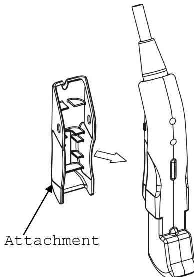
Fig. 5 How to attach the attachment
