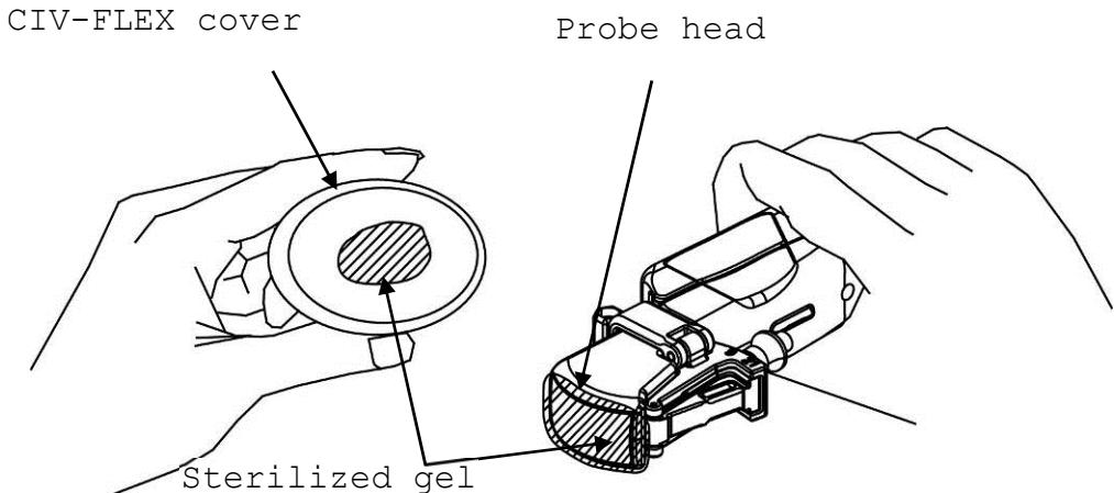
Fig. 13 Placing the gel
