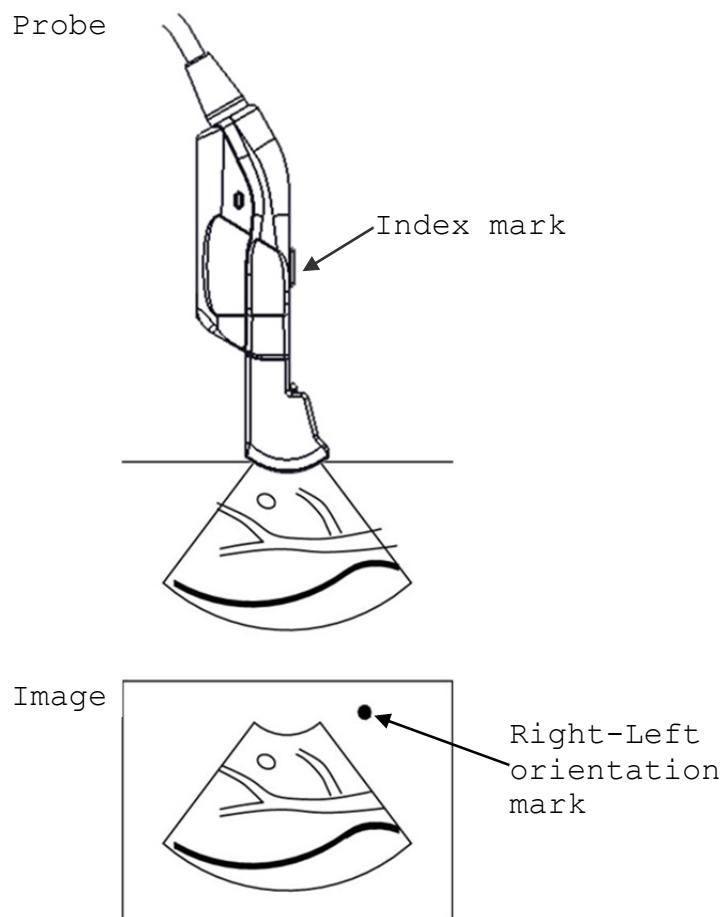
Fig. 4 Relationship between the directions of the probe and the Right-left orientation mark
