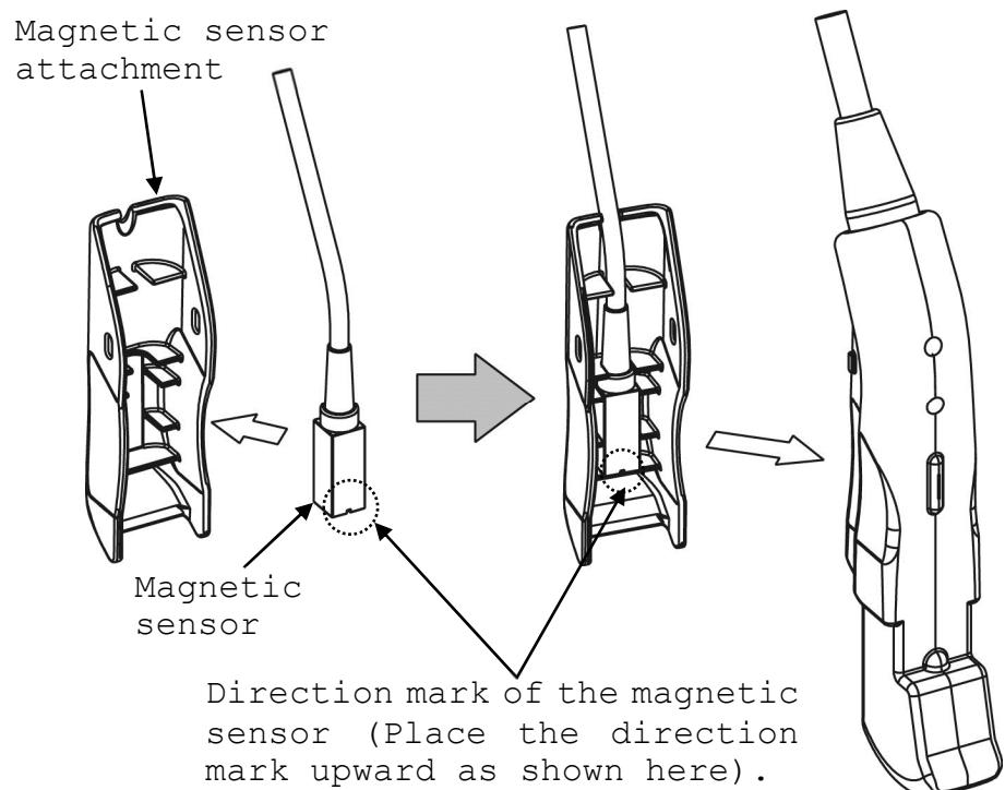
Fig. 7 How to attach the Magnetic Sensor Attachment
