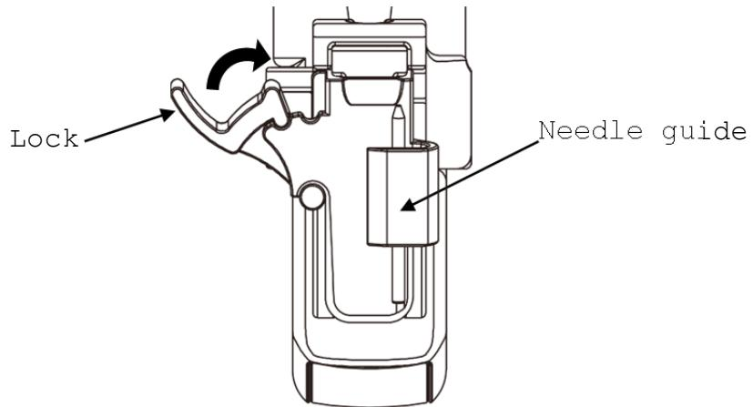
Fig. 15 Attaching the needle guide
