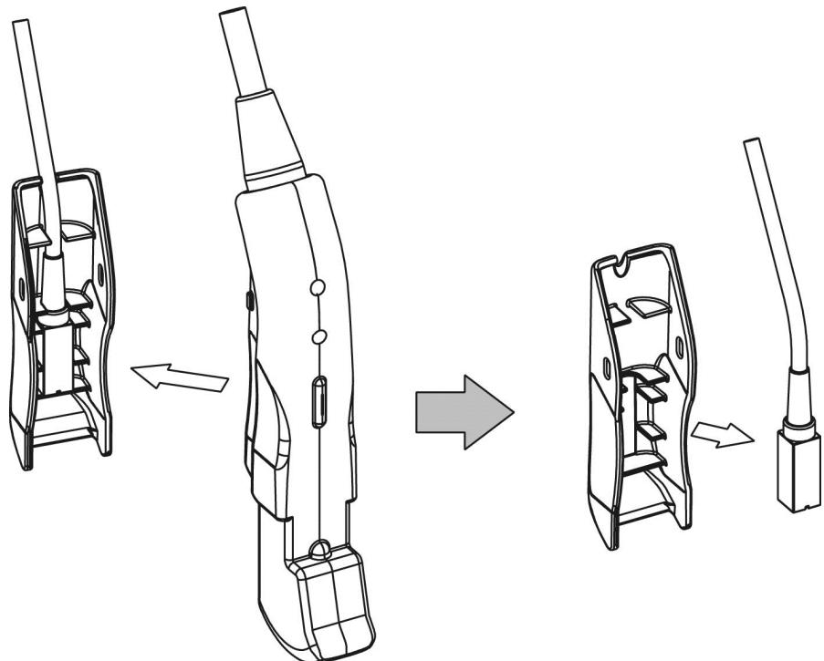
Fig. 9 How to release the Magnetic Sensor from the groove of the probe
