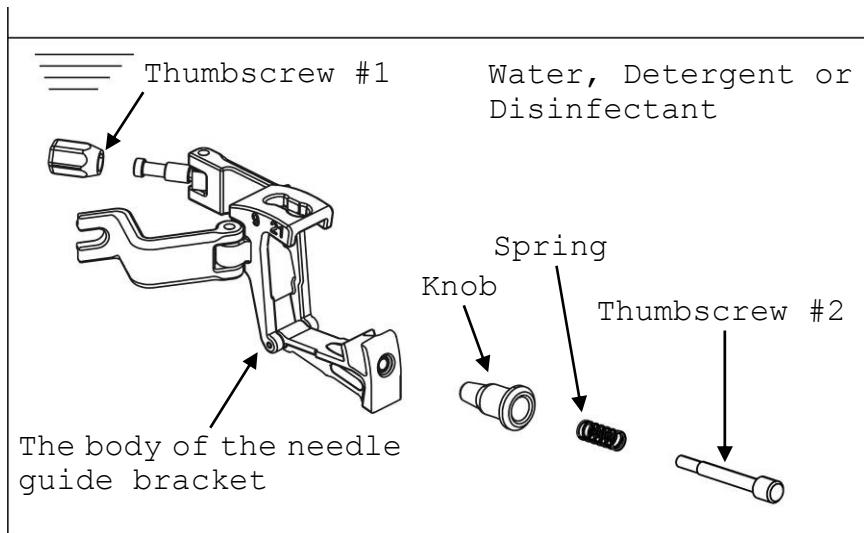
Fig. 22 Immersion of the Needle Guide Bracket
