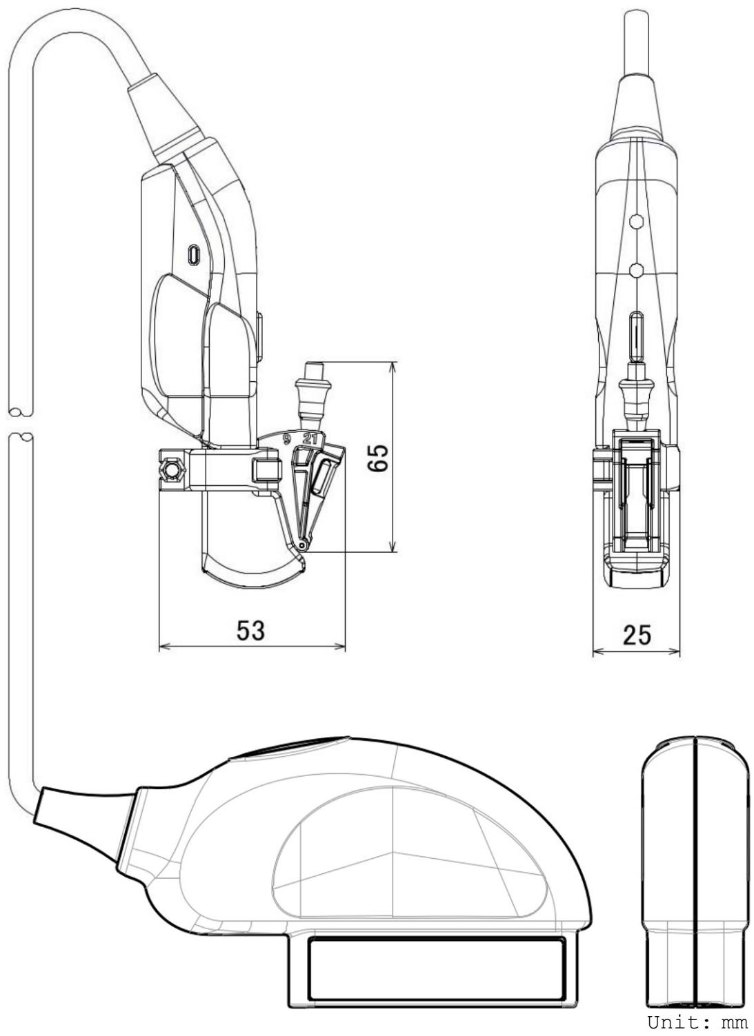
Fig. 25 Dimensions (with the Needle Guide Bracket)
