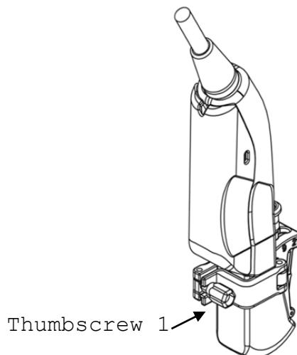
Fig. 12 Fitting the needle guide bracket
