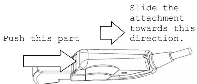
Fig. 6 How to release the attachment
